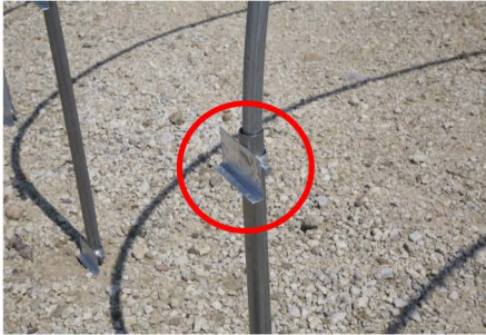
13. Attach Top Wood Adapter Brackets
