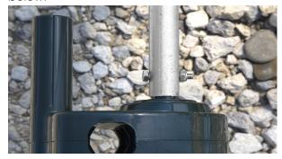
**Step 4:** Now that your greenhouse sidewall EMT conduit is attached to your crank, and the guide EMT conduit is properly installed, you can take your crank and slide it down to where the sidewall EMT conduit meets the guide EMT conduit. From there, simply turn your crank and watch as the crank lifts your greenhouse sidewall!
